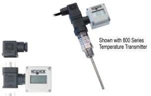
To install, remove the DIN 43650A plug and insert indicator on top of transducer and reinstall the plug. This indicator can be used with NOSHOK and some competitive transmitters with 2-wire 4 mA to 20 mA output, Hirschmann connector with the same pin configuration. (Pin 1 + supply, pin 2 + output)
